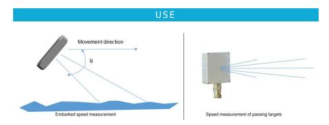
The waves emitted by the radar are always perpendicular to the antenna. Hence the two recommended installation positions for the sensor, according to the use are :
